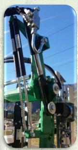
Cylinder for lifting the straddle bar
