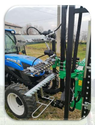
Model CL200 Scavallata adaptable for pruning of single curtain system with selfsharpening single-blade
