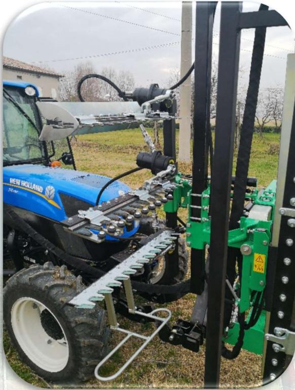
Model CL200 Scavallata adaptable for pruning of single curtain system with self-sharpening single-blade
