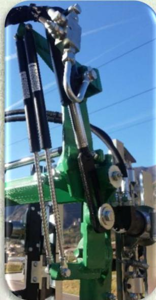
Cylinder for lifting the straddle bar
